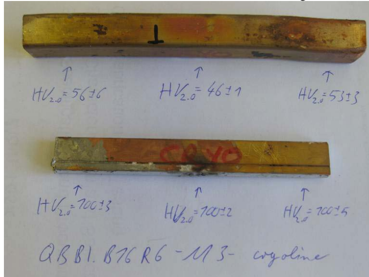
Figure 9: U-piece and wedge disconnected from LHC interconnection QBBLB16R6-M3-cryoline with Vickers indent positions. In the U-piece there is a significant hardness increase from the center to the extremities, due to a temperature gradient during soldering. After the HT for splice connection and disconnection, the wedge is still strongly cold worked.
