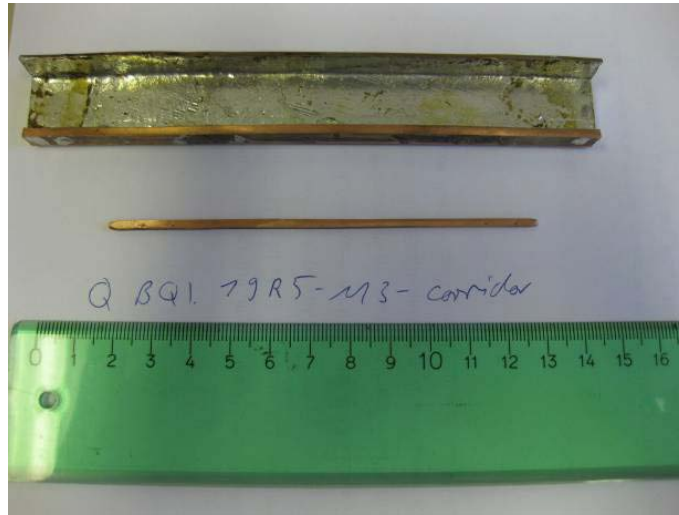
Figure 2: RRR sample machined out of U-piece disconnected from a LHC main bus bar splice.
