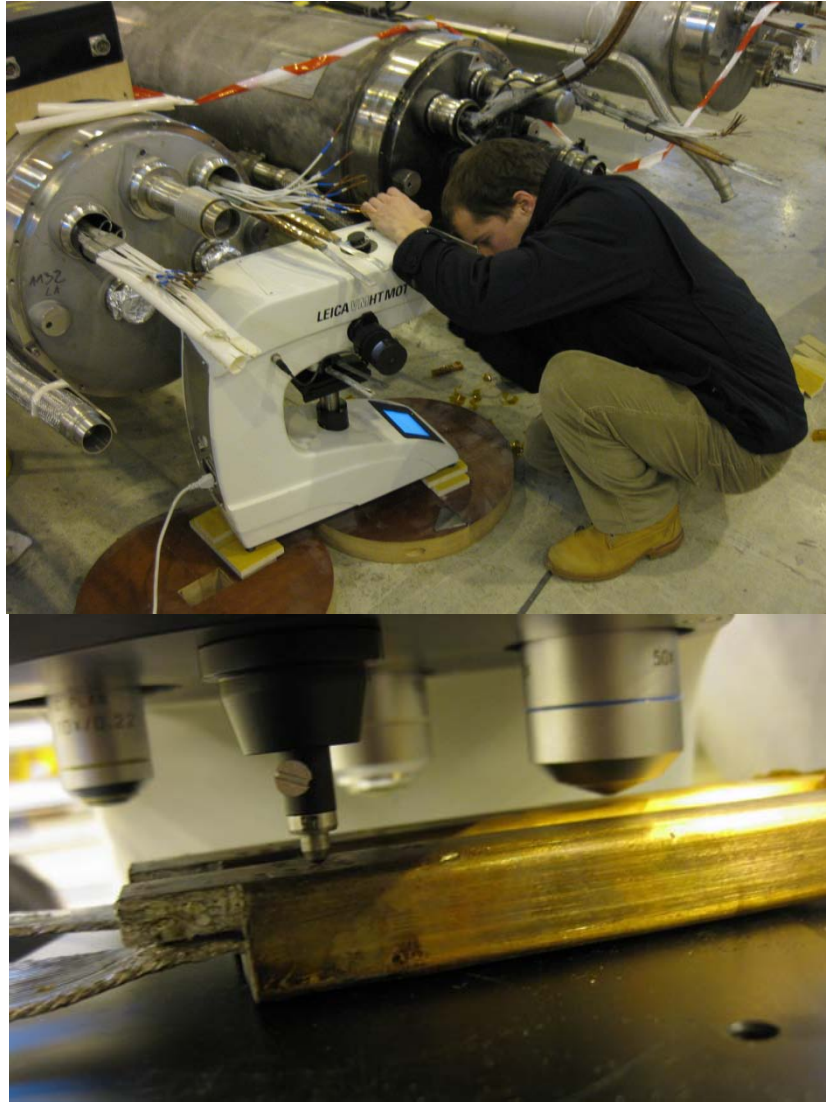
Figure 14: Vickers hardness measurements of the main dipole bus bar stabiliser in the LHC cryodipole 1132.
